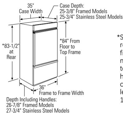
\*Shipping Height. The refrigerator can be adjusted to fit into a cutout that is 83-1/2" min. to 84-1/2" max. height. The top case trim at the front is 1/2" higher and will overlap upper cabinetry or soffit. Use leveling legs and wheels for a maximum 1" height adjustment.
