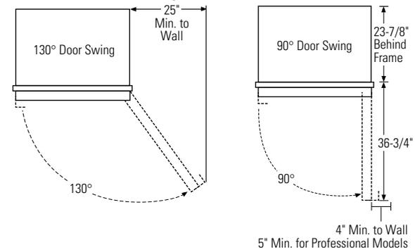
Allow 25" minimum clearances for a full 130° door swing. Allow 15" for pan removal.
