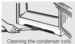
Cleaning the condenser coils.
