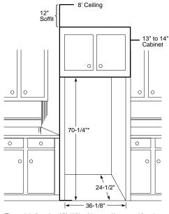
\*The rough-in dimension of 70-1/4\* is minimum and is measured from the finished floor to top of opening (or the underside of the overhead cabinets). For Models with Trim Kit: frameless style cabinets are planned for above the refrigerator, you may need to consider adding a maximum of 1/4\* (70-1/2\*) to height of opening to allow additional clearance between cabinet doors and top of refrigerator trim when cabinet doors are in open position.
