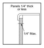
All other dotted lines indicate areas that must be routed out about 5/32" (4 mm) on the back side of panels 1/4" (6 mm) thick or more. For panels less than 1/4" (6 mm) thick, these areas can be cut out of the filler panel.
