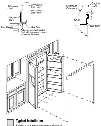
Shaded areas represent front surfaces of side panels and overhead cabinet or soffit that contacts trim.
