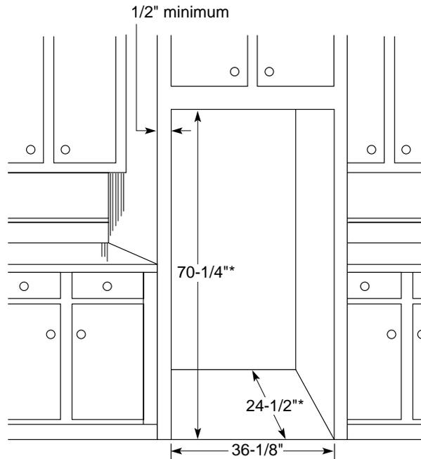
\*The rough-in dimension of 70-1/4" is minimum and is measured from the finished floor to top of opening (or the underside of the overhead cabinets). For Models with Trim Kit: If frameless style cabinets are planned for above the refrigerator, you may need to consider adding a maximum of 1/4" (70-1/2") to height of opening to allow additional clearance between cabinet doors and top of refrigerator trim when cabinet doors are in open position.
