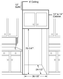
\*The rough-in dimension of 70-1/4\* is minimum and is measured from the finished floor to top of opening (or the underside of the overhead cabinets). For Models with Tim Kit: If frameless style cabinets are planned for above the refrigerator, you may need to consider adding a maximum of 1/4\* (70-1/2\*) to height of opening to allow additional clearance between cabinet doors and top of refrigerator trim when cabinet doors are in open position.
