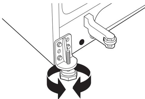
**⚠ CAUTION:** To avoid possible personal injury or property damage, the leveling legs must be firmly touching the floor.
