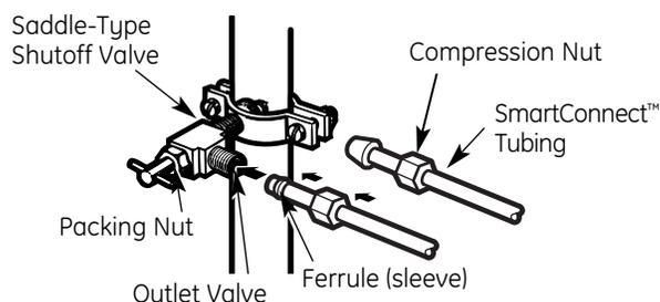
**NOTE:** Commonwealth of Massachusetts Plumbing Codes 248CMR shall be adhered to. Saddle valves are illegal and use is not permitted in Massachusetts. Consult with your licensed plumber.
