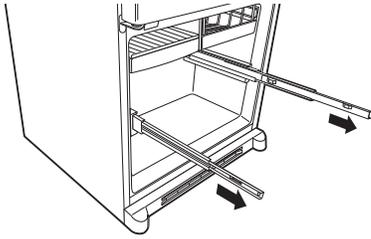
**B** Locate the slots on the inside of the rail assemblies near the back.
