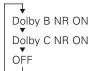
The B NR indicator lights up when Dolby B NR is turned on, and the C NR indicator when Dolby C NR is turned on.
