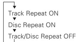
"Track Repeat ON/T-Repeat ON" is displayed and the track number blinks in the display when track repeat is on.
