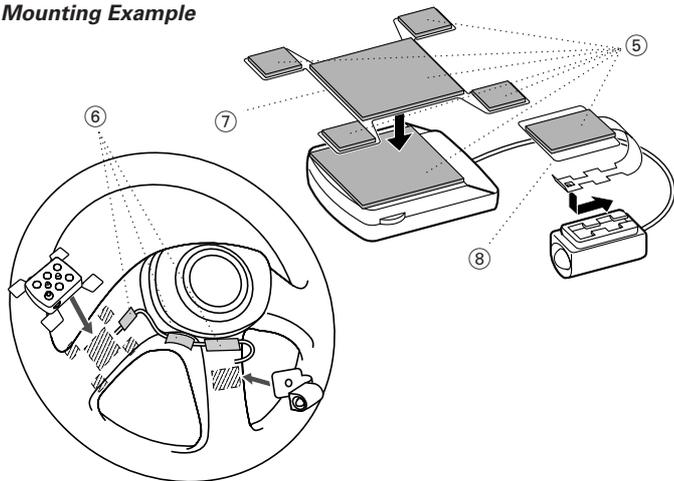
Attach the operation section and the light emitting section of the Steering Remote Control as shown above. Be sure to attach them to positions that can ensure proper operation.
