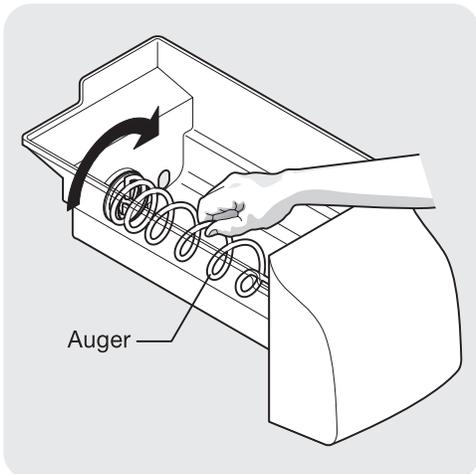
**IMPORTANT:** When removing or replacing the ice bin, do not rotate the auger in the ice bin. If the auger is accidentally turned, you must realign the auger by turning it in 90° turns until the ice bin fits into place with the drive mechanism.
