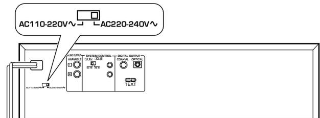
Move switch lever to match your line voltage with a small screwdriver or other pointed tool.
