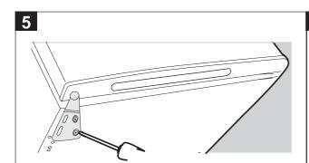
Screw the two screws to install the top bracket on top right side of appliance. Slide the appliance door back on to the top hinge. Making sure it's face up. Then replace the "plastic cover" on the top bracket by clicking back into position of door hinge.
