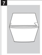
Check that the door is aligned horizontally and vertically and that the seals are closed on all sides before finally tightening the bottom hinge. Re-adjust the leveling feet.
