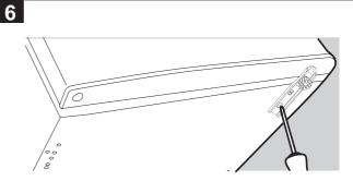
Screw the bottom hinge into place on the new side. Replace the other foot on the other side.
