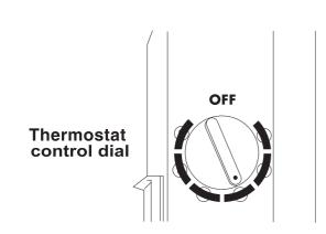
The thermostat for the refrigerator is located at the upper right hand corner of the refrigerator compartment.
