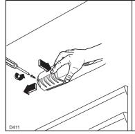
**2.** Replace the light cover by sliding it into its original position and replacing the screw.
