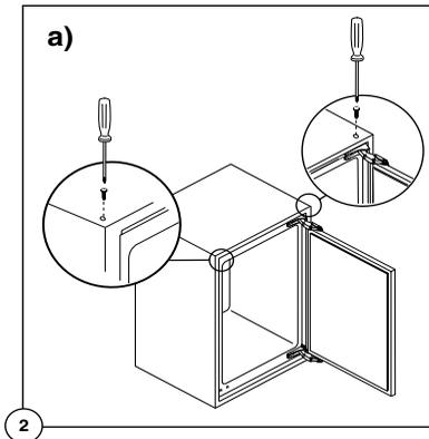
2. Position the two brackets as shown in the figure and replace the two securing screws.
