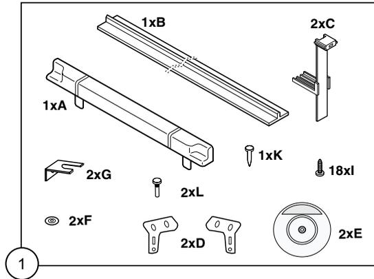
Two cabinet securing brackets are supplied with the installation pack. They need to be assembled onto the cabinet prior to cabinet being pushed into the Kitchen aperture.
