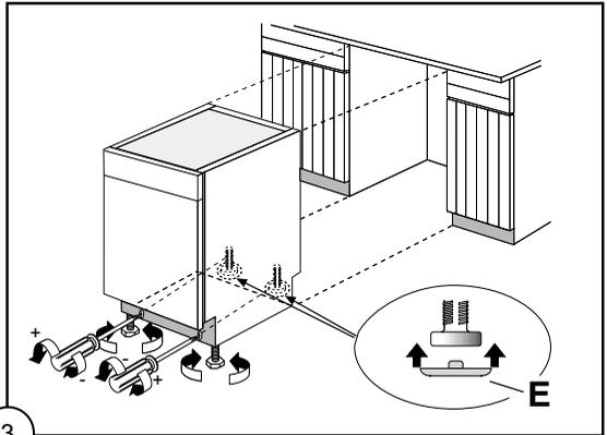
The rear feet are adjusted by turning the screw in the front kick plate to the left or right.
