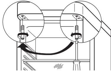
6. Carefully slide the door onto the top bearing pivot and close.
