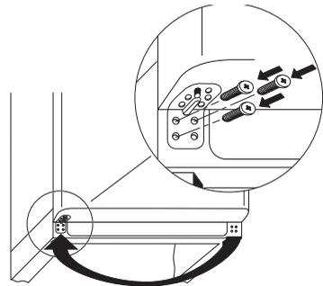
8. Move the door handle from the left to the right and cover the remaining holes with the blanking plugs attached.
