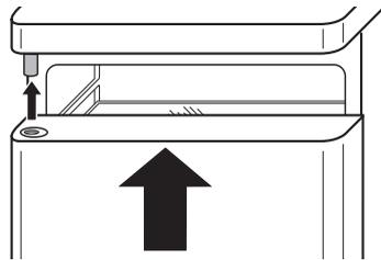
7. Place the lower door bearing with the bearing pivot in the lower left of the door and fasten.
