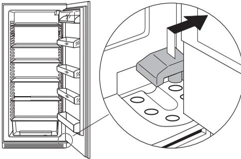
3. Wash the inside of the appliance with lukewarm water with a little bicarbonate of soda added (5 ml to 0.5 litre of water). Do not use soap or detergent as the smell may linger. Dry the appliance thoroughly. Remove the transport fittings from the storage shelves:
