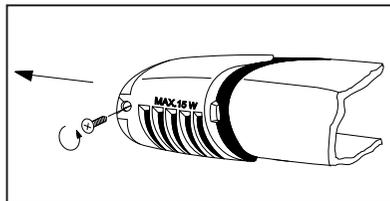
After changing the bulb replace the lamp cover, and retaining screws and reconnect the appliance to the electricity supply.
