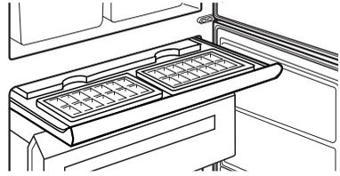
**i** In the event of power failure or a malfunction of the appliance, the cold accumulation block will increase the hold over period by several hours.
