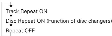
"Track Repeat ON"/"Repeat ON" is displayed and the track number blinks in the display when track repeat is on. "Disc Repeat ON" is displayed and the disc number blinks in the display when disc repeat is on.
