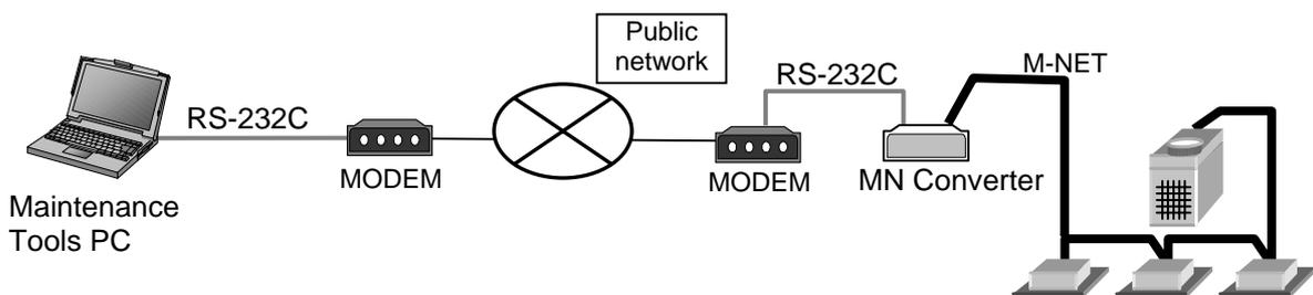
\*For the remote connection utilizing MN Converter, an isolator is required to be inserted between the modem and MN Converter.
