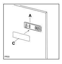
Open the appliance door and the furniture door at  $90^{\circ}$ . Insert the small square (B) into guide (A). Put together the appliance door and the furniture door and mark the holes as indicated in the figure. Remove the squares and drill holes with  $\emptyset$  2 mm at 8 mm from the outer edge of the door. Place the small square on the guide again and fix it with the screws supplied.
