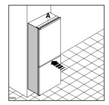
For a correct alignment make sure that the distance between the appliance and the cabinet is of 44 mm.
