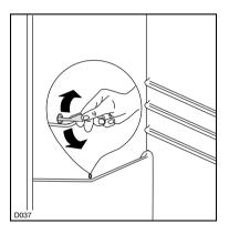
It is important to periodically clean the defrost water drain hole in the middle of the refrigerator compartment channel to prevent the water overflowing and dripping onto the food inside. Use the special cleaner provided, which you will find already inserted into the drain hole.
