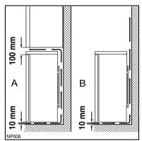
There should also be a gap of 25 mm either side of the appliance. Do not obstruct the space underneath. The back of the cabinet may be placed close to the wall but must not touch it. DO NOT install in places with restricted ventilation. Adjust the level of the appliance by screwing out the adjustable foot, or feet, at the bottom of the cabinet using your fingers.
