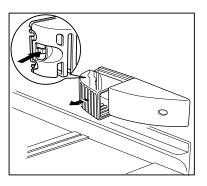
press on the rear hook and at the same time slide the cover in the direction indicated by the arrow. Unscrew the bulb and replace it with one of the same power (the maximum power is shown on the light diffuser) available from your nearest Service Force Centre.
