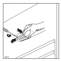
Unscrew the light cover and then pull it outward by pressing as shown in the figure. Unscrew the bulb and replace it with a new 15 watt bulb (available from your nearest Electrolux Service Force Centre).
