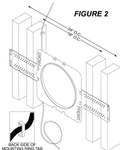
**Step 2.** After you have determined the speaker locations using the guidelines above, secure a 16 gauge 2 - c o n d u c t o r cable to the mounting ring tabs (see figure 2), such as the M&S Systems MS 16 X, for attachment to the speakers after the dry wall has been
