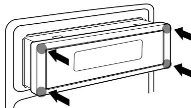
▲ To attach this unit, make sure the front of the control panel faces you and fit it into the mounting sleeve by pressing the four corners of the hard rubber frame at the same time.
