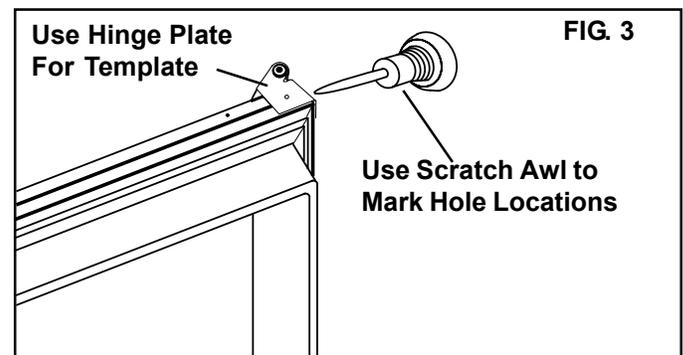
5. Predrill three 3/32" holes into the door hinges as marked in step 4.
