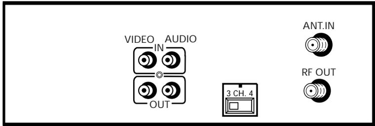
**3 CH. 4 Switch** Selects the channel to which you will tune the TV to see the VCR picture if you connect the VCR using the ANT.IN and RF OUT jacks.
