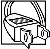
Caution: To reduce the risk of electric shock, match wide blade of plug to wide slot, fully insert.
