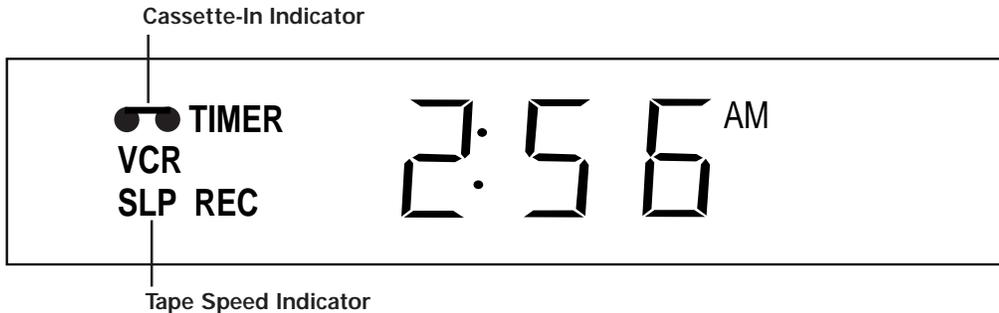
Cassette-In Indicator (
