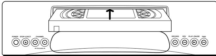
If the Auto Play feature is set to ON, the tape automatically begins playback (if the safety tab on the cassette is removed).
