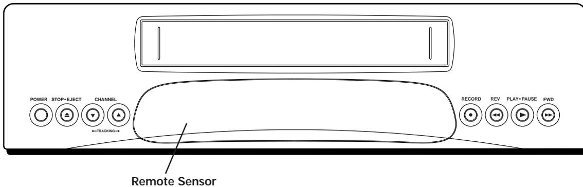
**CHANNEL•TRACKING** Up or Down Selects next higher or lower channel in the VCR's channel memory. Adjusts tracking when a tape is playing.
