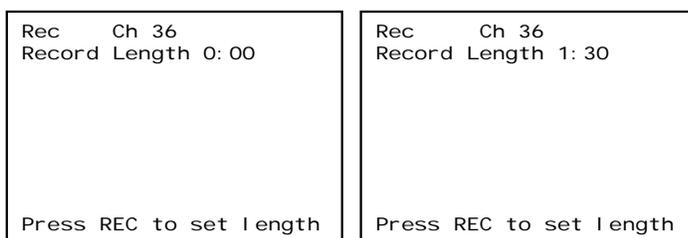
Each press of the RECORD button increases the recording time (up to 4 hours).
