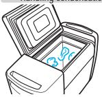
Condensation will form on the product during operation. Quickly wipe any moisture that forms on the main unit, or drips out of the cooler.
