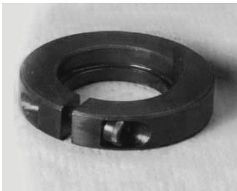
Fig. 7 - Tightening Locking Collar
