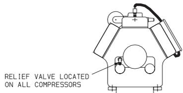
RELIEF VALVE LOCATED ON ALL COMPRESSORS
