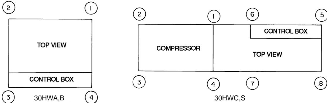
WEIGHT DISTRIBUTION AT EACH MOUNTING HOLE — Lb (kg)
