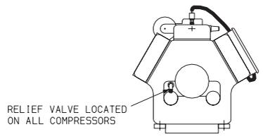
RELIEF VALVE LOCATED ON ALL COMPRESSORS
