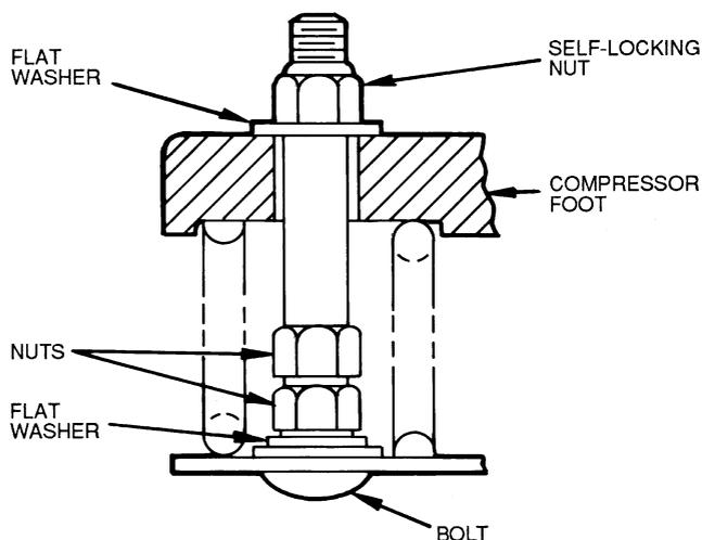
**Fig. 12 — Compressor Mounting**
