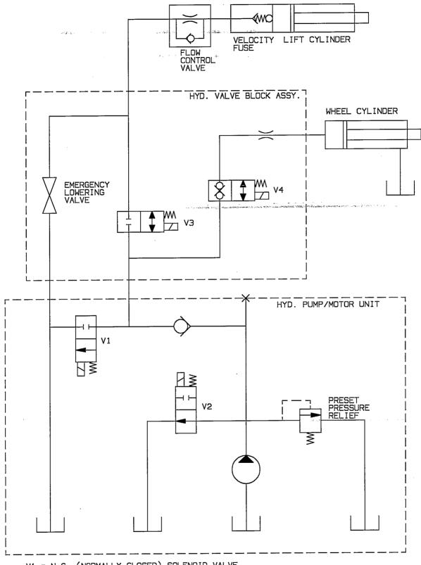
V1 = N.C. (NORMALLY CLOSED) SOLENOID VALVE V2 = N.O. (NORMALLY OPEN) SOLENOID VALVE V3 = RAISE/LOWER SOLENOID VALVE V4 = WHEEL RAISE/LOWER SOLENOID VALVE
