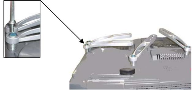
1. Locate the mounting points on the bottom of the projector (see arrows above for mounting point recognition).
