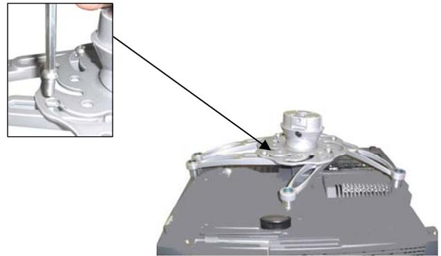
4. Align the projector plate to the mounting legs.
