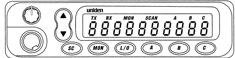
**Microphone Jack** - Allows attachment of standard, DTMF or base station microphone.
