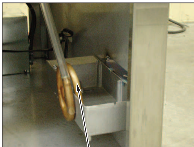
Drain Pan Heater - PN-27799
