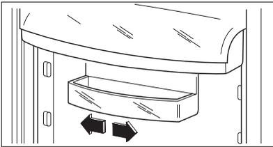
The model is equipped with a variable storage box which is fitted under a door shelf compartment and can be slide sideways.
