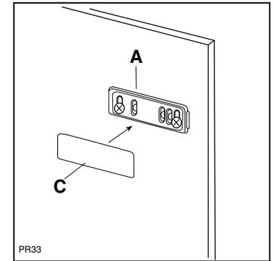
Open the appliance door and the furniture door at 90°. Insert the small square (B) into guide (A). Put together the appliance door and the furniture door and mark the holes as indicated in the figure. Remove the squares and drill holes with  $\varnothing 2$  mm at 8 mm from the outer edge of the door. Place the small square on the guide again and fix it with the screws supplied.
