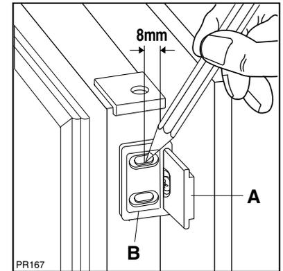
At the end of installation/adjusting, it is necessary to check if the door of the furniture closes properly. Should adjustment of the furniture door be necessary, use the clearance of slots.
