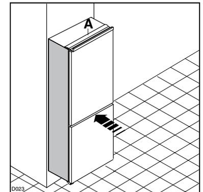
Open the door and push the appliance against the side of the kitchen unit opposite to that of appliance hinges.
