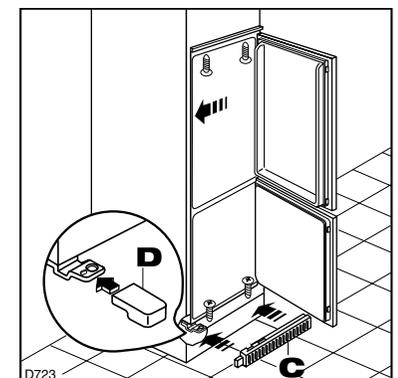
1. Unscrew the upper pin and remove the spacer
