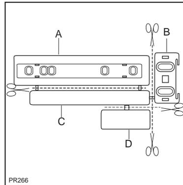
Place guide (A) on the inside part of the furniture door, in the upper and lower positions as shown in the figure and mark the position of external holes. Having drilled the holes, fix the guide with the screws supplied.
