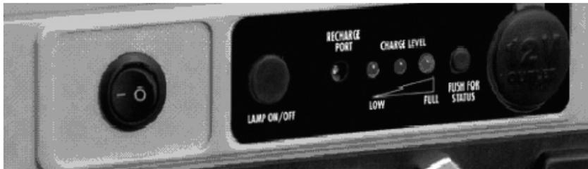
The **VEC270MG** can be recharged from any standard 120 volt AC power source using the supplied AC recharge adapter. The adapter's barrel connector attaches to the recharge port on the side panel.
