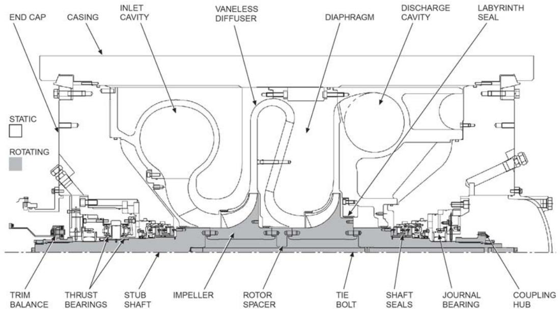
**Figure 7. Cross Section of a Solar Gas Compressor**
