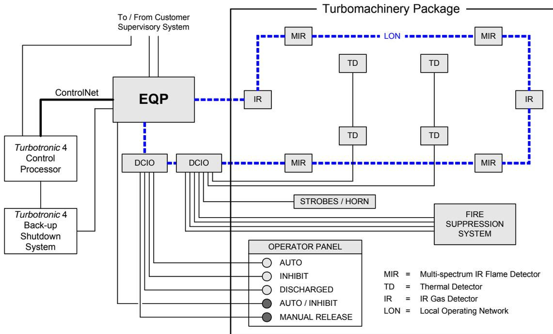
**Figure 21. Typical Fire and Gas System**
