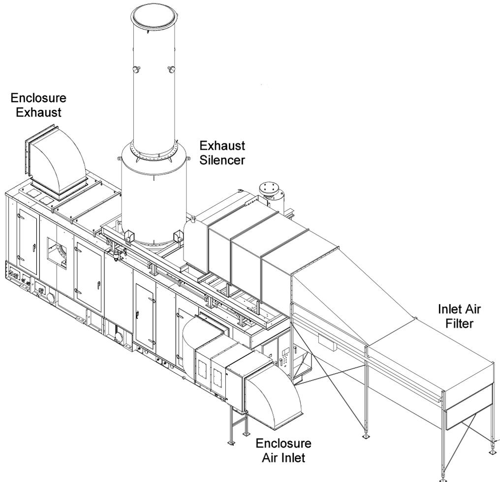
**Figure 24. Typical Enclosed Taurus 60 Package with Exhaust and Inlet Systems**
