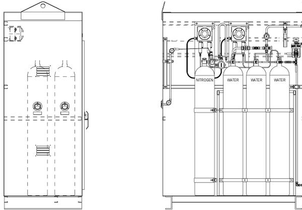
**Figure 23. Typical Water Mist Suppression Fire Cylinder Cabinet**
