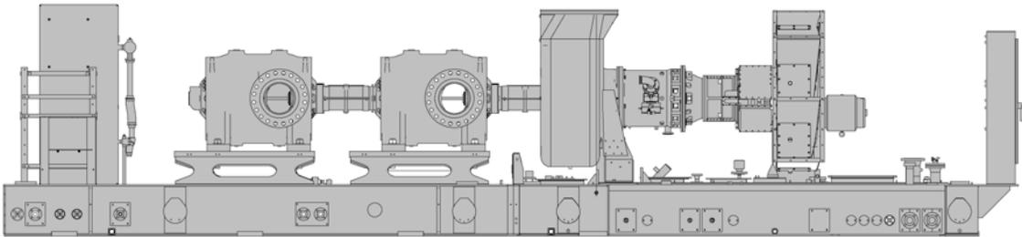
**Figure 5. Compressor Set with Taurus 60 Driving Tandem Solar Compressors**
