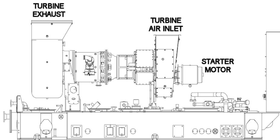
Figure 1. Typical *Taurus 60* Gas Turbine Mechanical Drive
