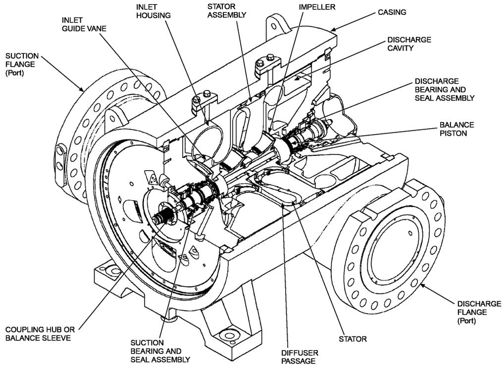
**Figure 6. Cutaway Diagram of a Solar Gas Compressor**
