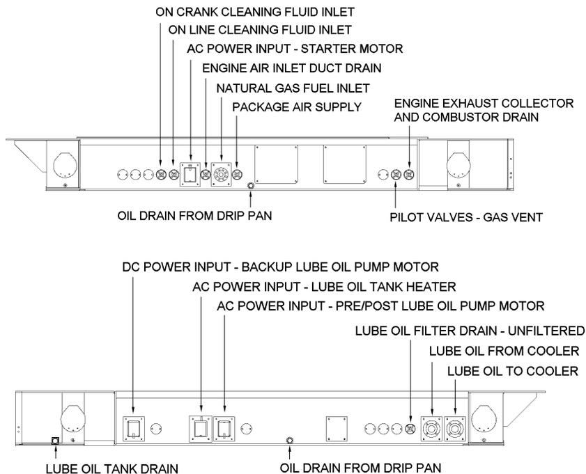
**Figure 2. Typical Taurus 60 Mechanical Drive Service Connections**
