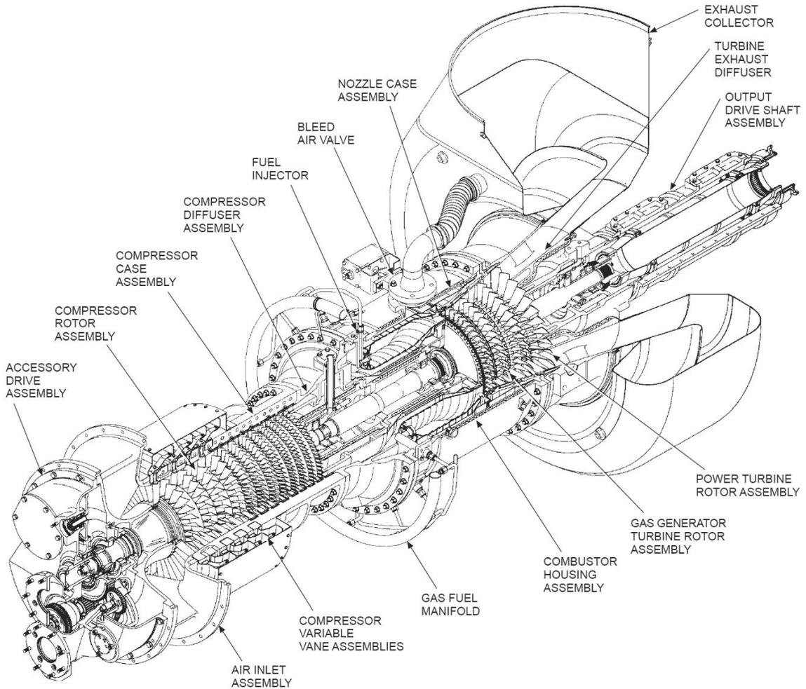
**Figure 3. Typical Taurus 60 Two-Shaft Gas Turbine**
