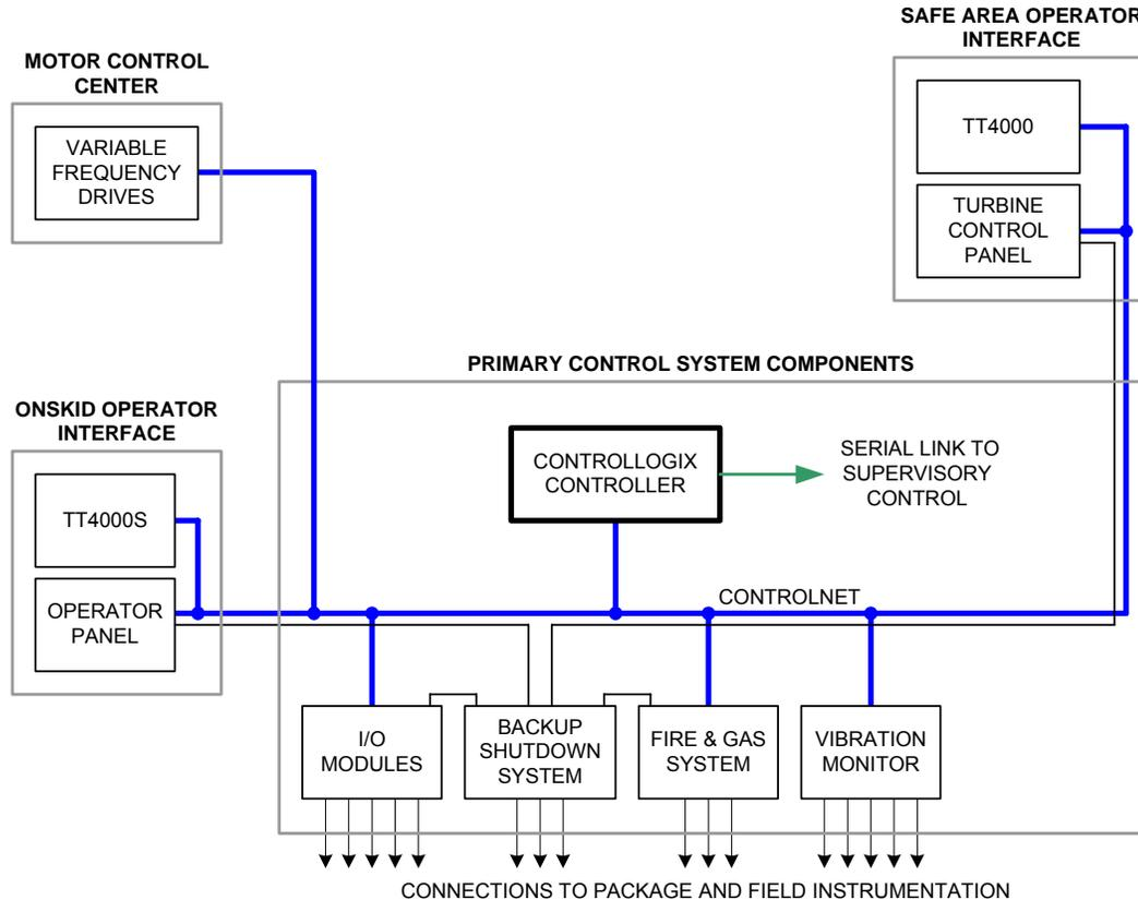
**Figure 16. Turbotronic System Architecture**
