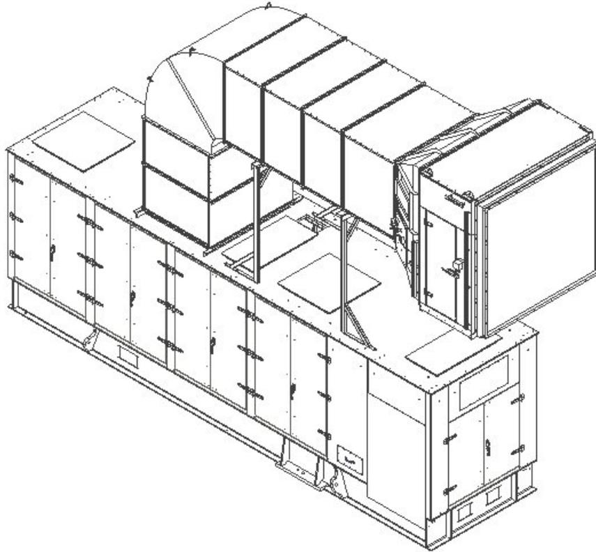
**Figure 26. Typical Taurus 60 Medium Velocity Air Inlet System**
