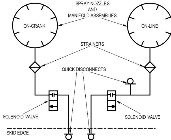
**Figure 28. Turbine Cleaning System**
