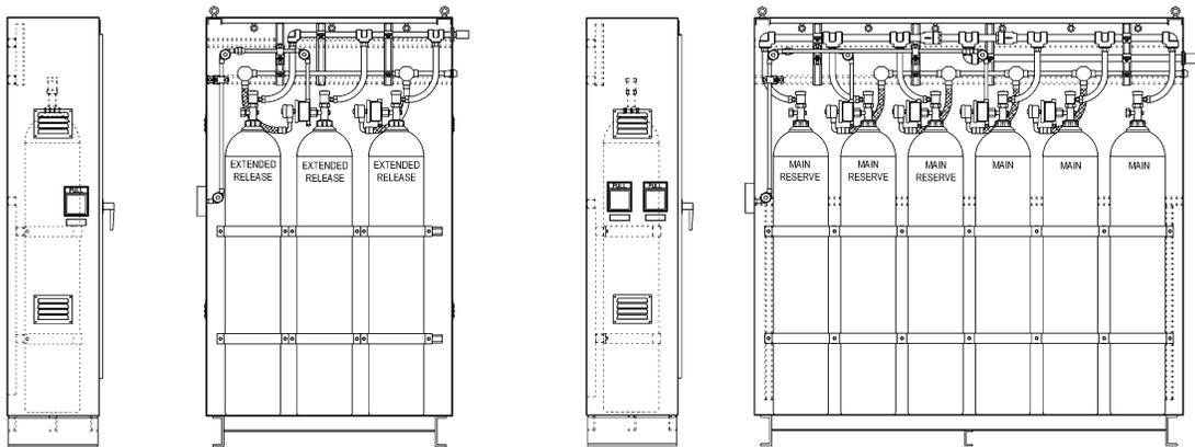
**Figure 22. Typical CO<sub>2</sub> Suppression Fire Cylinder Cabinets**
