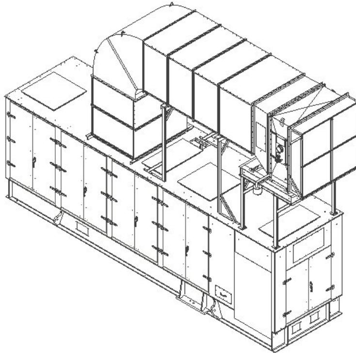
**Figure 25. Typical Taurus 60 High Velocity Air Inlet System**
