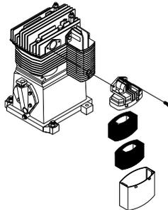
**AIR COMPRESSOR PUMP:** To compress air, the pistons move up and down in the cylinders. On the downstroke, air is drawn in through the air intake valves while the exhaust valves remain closed. On the upstroke, air is compressed, the intake valves close and compressed air is forced out through the exhaust valves, into the discharge line, through the pilot valve and into the air tank.
