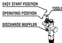
**SAFETY RELIEF VALVE:** This valve is designed to prevent system failures by relieving pressure from the system when the compressed air reaches a predetermined level. The valve is preset by the manufacturer and must not be modified in any way. To verify the valve is working properly, pull on the ring. Air pressure should escape. When the ring is released, it will reset.
