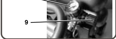
**9) PRESSURE REGULATOR:** The air pressure coming from the air tank is controlled by the regulator knob. Turn the pressure regulation knob clockwise to increase discharge pressure, and counterclockwise to decrease discharge pressure. Follow tool operating instructions for recommended pressure range.
