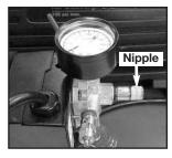
6. Assemble the regulator and orient as shown.
