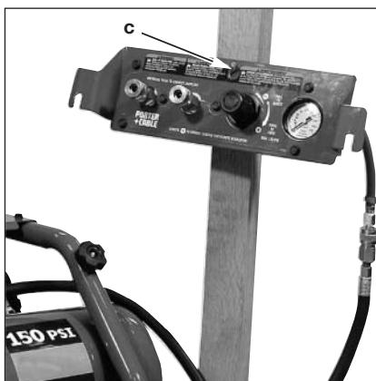
**WARNING** Can cause serious injury or death. Tank may contain 150 PSI of air pressure. Never connect accessories to unregulated air. Never operate tools or accessories above marked maximum pressure.
