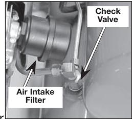
**Check Valve:** When the air compressor is operating, the check valve is "open", allowing compressed air to enter the air tank. When the air compressor reaches "cut-out" pressure, the check valve "closes", allowing air pressure to remain inside the air tank.
