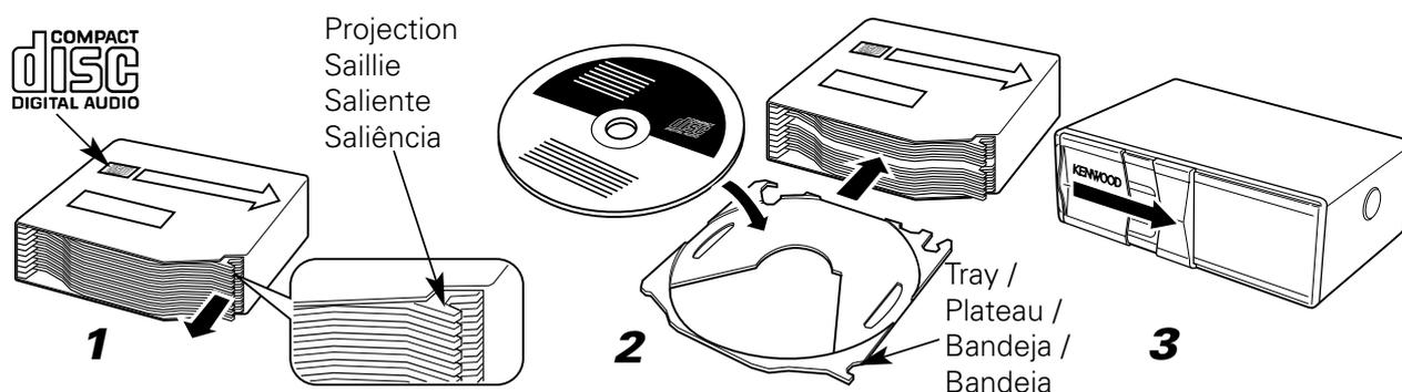
1. Make sure the disc magazine is the right way up with the "disc" logo on the top. Pull the tray out by the projection.
