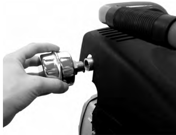
Figure 4. Installing the Air Filter
