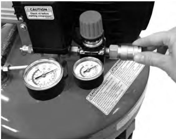
Figure 3. Installing the Air Chuck
