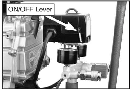
**Figure 9.** ON/OFF lever.
