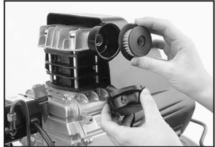
Figure 15. Air filter element.
