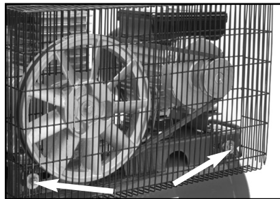
Figure 10. Belt Guard and mounting bolts.
