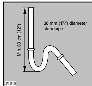
When discharging into a standpipe ensure that the top of the curve in the hose end is no more than 90cm (35.4") and no less than 60cm (23.6") above floor level.
