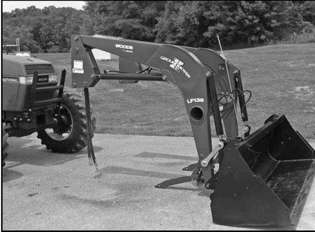
**Figure 44.** Align Tractor to Loader
