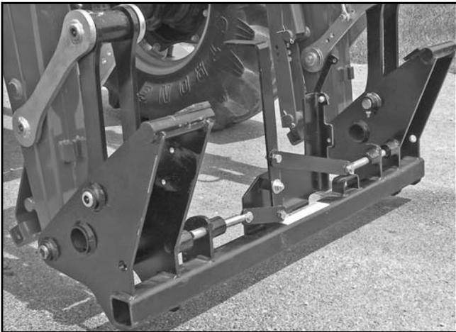
Figure 38. Quick Attach Coupler Installed
