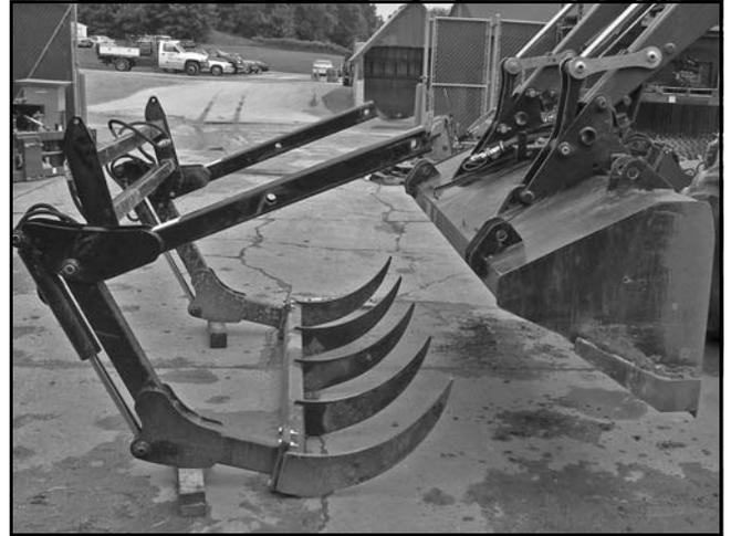
**Figure 50.** Align Bucket with Grapple
