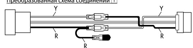
Use modified wiring 1 if the unit does not turn on.
