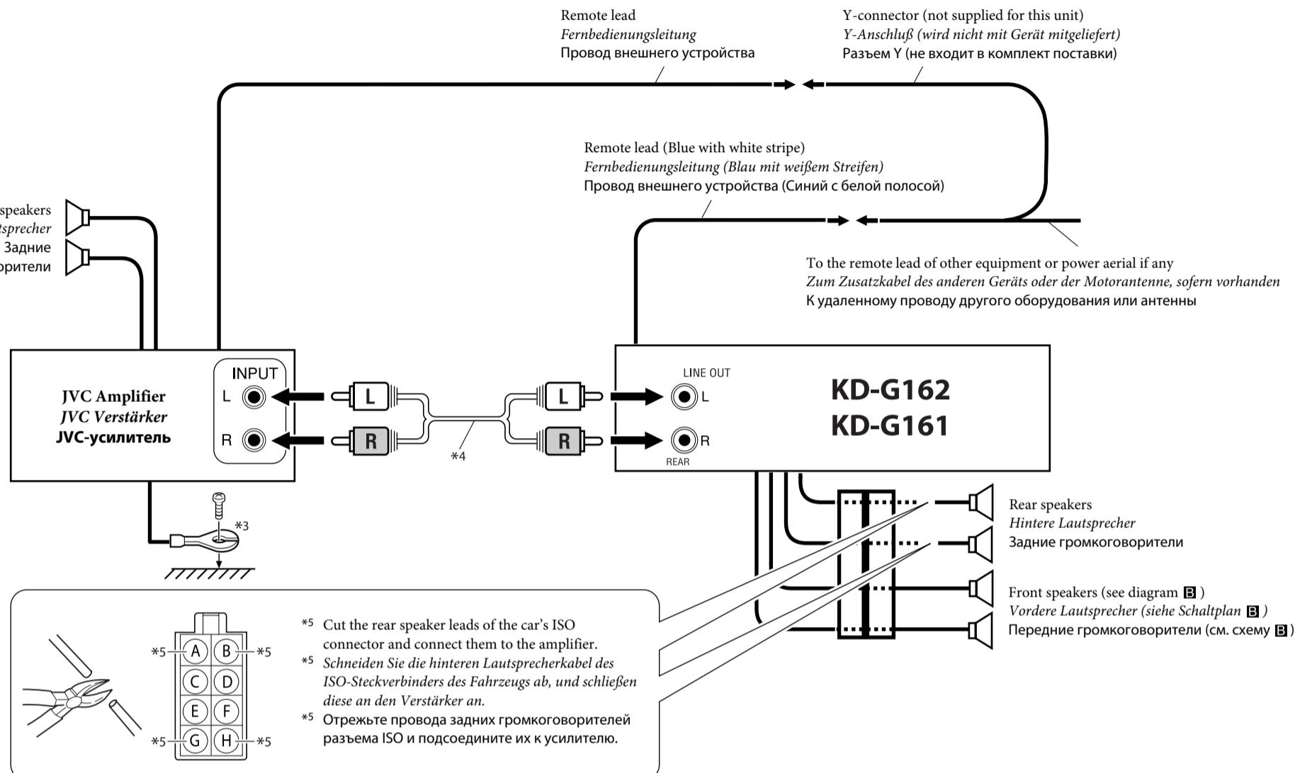
\*3 Firmly attach the ground wire to the metallic body or to the chassis of the car—to the place not coated with paint (if coated with paint, remove the paint before attaching the wire). Failure to do so may cause damage to the unit.
