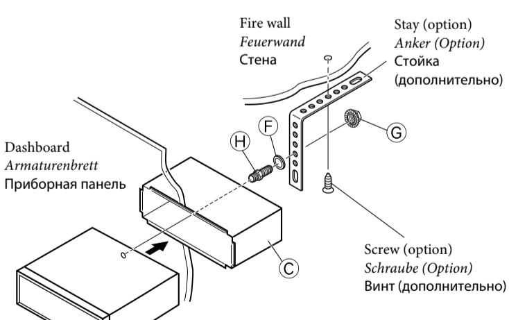
Install the unit at an angle of less than 30°.
