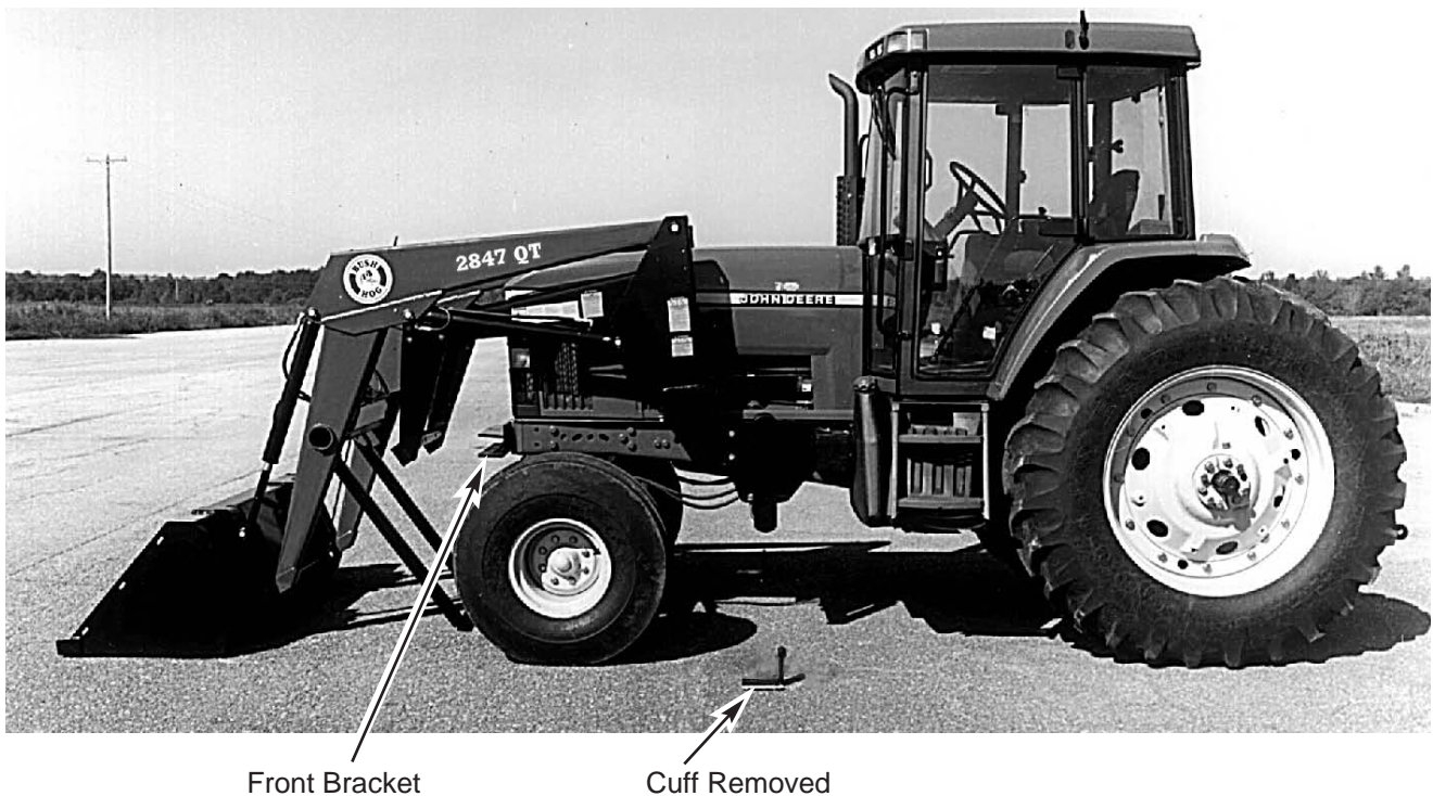
Figure 2-2 Drive In Close Enough To Allow Connecting Hydraulic Hoses To Tractor Outlets
