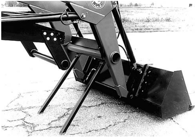
Figure 5-1 Parking Stands Installed
