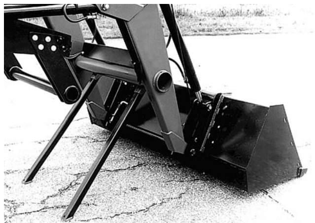
Figure 2-7 Parking Stands Installed
